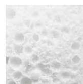
HOK Mixture of spherical al- uminium oxide
