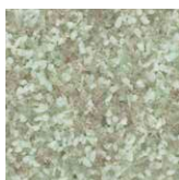
CERAMIC Ceramic grain and monocrystal aluminium oxide
